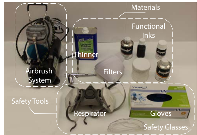
Figure 2. Our hardware setup includes an airbrush, functional inks, and safety tools.
