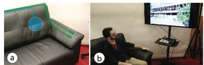
Figure 14. Interactive sofa. (a) A touch sensor (blue) detects if a users sits on the sofa. Two proximity sensors (green) sense swipe gestures. (b) A photo album app starts when a user sits down. Swiping over the armrest switches through photos.
