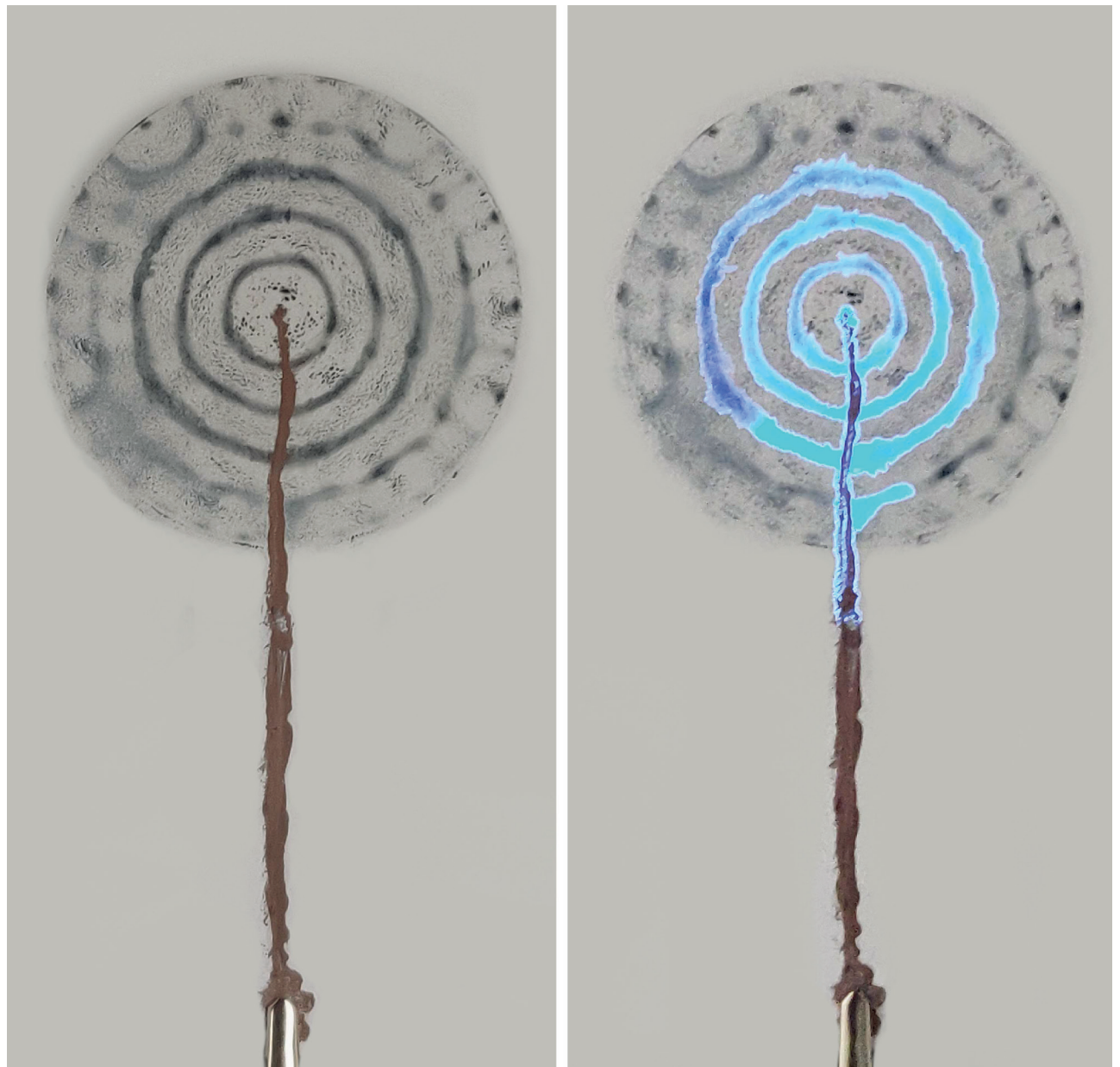
Fig. 15: Sonolithographs made with active materials in off and on states.
