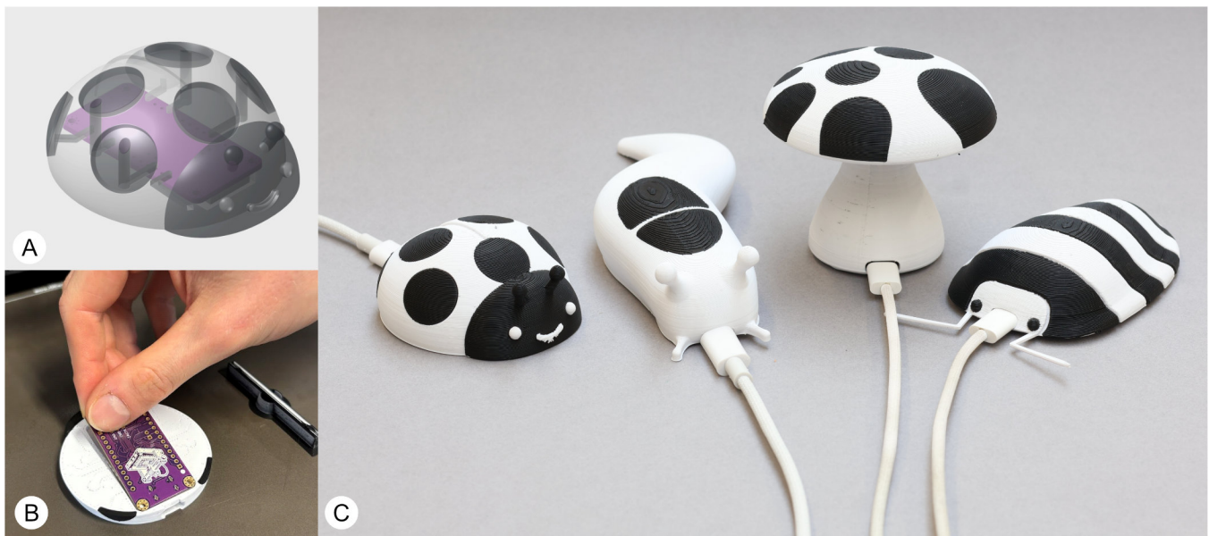
Figure 1: Printegrated Circuits is a new approach that leverages multi-material 3D printers to create seamless interactive objects with embedded circuitry. (A) Interactive objects are designed with conductive elements and traces with cavities for embedded PCBs (B). During fabrication, the 3D printing process is paused to allow PCBs to be inserted inside an object. (C) Four example Printegrated Circuit designs that detect touch interactions and communicate over USB.
