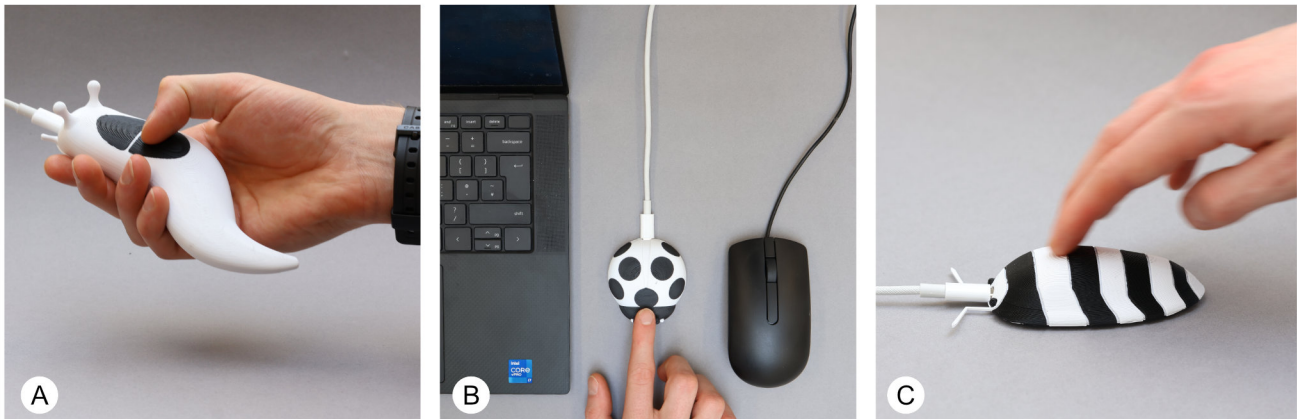
Figure 12: The slug, ladybird and isopod are all USB HID devices derived from the same base functional design, but each is customised to have a unique form and function. (A) the slug is a haptic presentation clicker, (B) the ladybird is a media controller, (C) the isopod is a stroke-sensitive desk pet.
