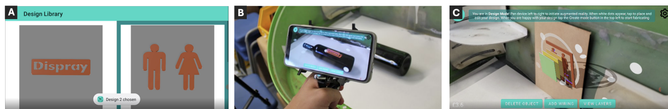
Figure 6: The design mode of the Dispray system showing: A) the design library where a user can pre-select an electrode layout; B) the upload of the template to AR, shown as a logo that is superimposed onto a physical object, to be used as a virtual template; C) The visualization of layers over a design before any spraying happens.
