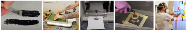
Figure 11: Fabrication methods for active material deposition and layering related work: Paintbrush and craft-based methods (shown here is conductive BareConductive paint [29]) used in display fabrication - Kaihou et al. use this process for TC materials [84], screen printing [75], inkjet printing [134], hydrodipping [82] and spraying [207]. All images copyright maintained by original owners: ACM
