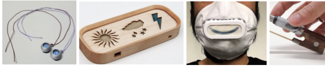
Figure 8: Research projects exploring both electrochromic and electrophoretic personally fabricated displays for information conveyance. Always with me [74], Ambient display design space [126] and EC facemask [47] as well as an exploration of E ink fabrication within FabricatINK [54]. All images copyright maintained by original owners: ACM
