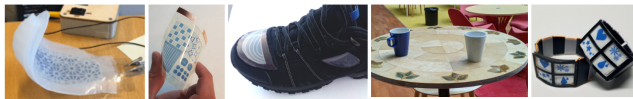
Figure 7: Research projects exploring electrochromic personally fabricated displays: Chromabot [15], Transprint [75], EC running shoe [128], Cleanleaf [25], Always with me [74]. All images copyright maintained by original owners: ACM
